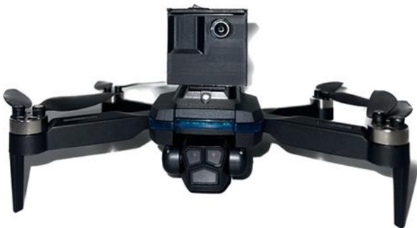
Fig. 5. Smart thermal imaging drone.
