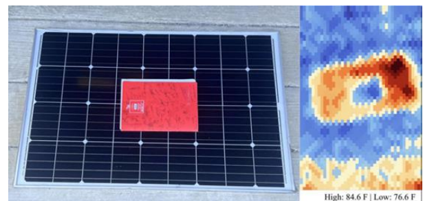
Fig. 7. Subsequent test for shadow case.
